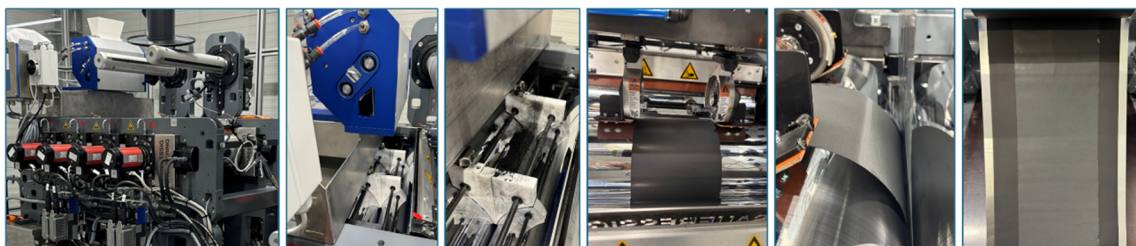
Figure 18: Images taken during the dosing process with the roller feeder from Coperion K-Tron, as well as during the film formation and lamination process with the ProLiT calender from Saueressig/ Matthews Engineering (created by M. Nickl)
