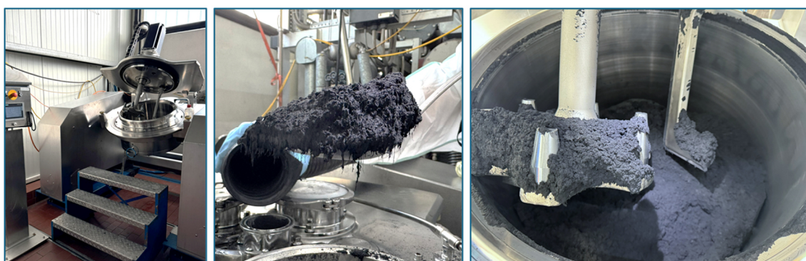
Figure 16: Shown are images taken during the batch mixing process in a 50-liter Eirich mixer at Maschinenfabrik Gustav Eirich GmbH & Co. KG.
